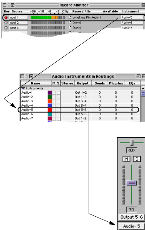
Figure 10.3: Typical audio recording setup
