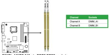
P5KPL-AM/PS 240-pin DDR2 DIMM sockets
