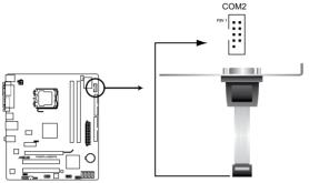
P5KPL-AM/PS Serial port (COM2) connector
