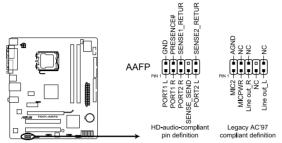
P5KPL-AM/PS Analog front panel connector
