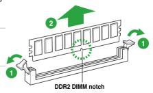
2. Remove the DIMM from the socket.
