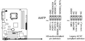
P5QPL-AM Analog front panel connector
