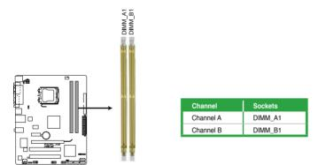
P5QPL-AM 240-pin DDR2 DIMM sockets
