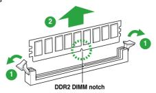
Remove the DIMM from the socket.
