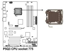
Before installing the CPU, make sure that the cam box is facing towards you and the load lever is on your left.
