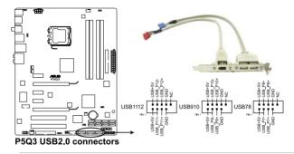
Never connect a 1394 cable to the USB connectors. Doing so will damage the motherboard!
