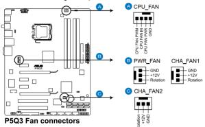
DO NOT forget to connect the fan cables to the fan connectors. Insufficient air flow inside the system may damage the motherboard components. These are not jumpers! DO NOT place jumper caps on the fan connectors!
