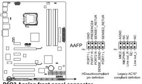
P5Q3 Analog front panel connector
