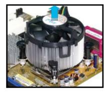
Rotate each fastener clockwise to ensure correct orientation when reinstalling.
