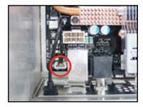
This photo shows the LCD Poster installed. Place the device wherever you can monitor the screen.
