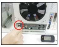
Plug the LCD Poster cable into the onboard connector labeled LCD\_CON.
