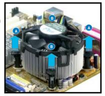
Carefully remove the heatsink and fan assembly from the motherboard.
