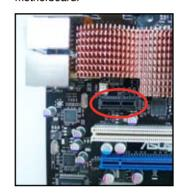
Align the card connector with the slot and press firmly until the card sits on the slot completely.
