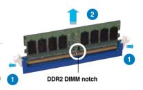
2. Remove the DIMM from the socket.
