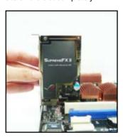
The photo below shows the audio card installed on the motherboard.
