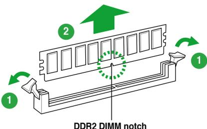
2. Remove the DIMM from the socket.
