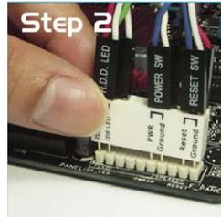
When installed, the Q-connector appears as shown.
