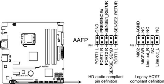
**P5Q-EM DO Analog front panel connector**
