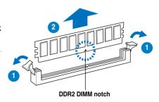
2. Remove the DIMM from the socket.
