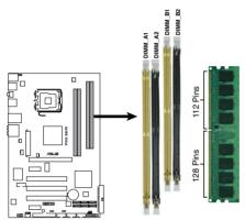
P5Q SE/R 240-pin DDR2 DIMM Sockets
