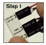
Install the ASUS Q-Connector to the system panel connector, ensuring the orientation matches the labels on the motherboard.
