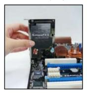
2. Locate the audio slot on the motherboard.
