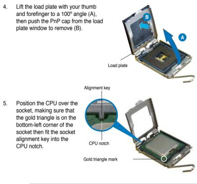
The CPU fits in only one correct orientation. DO NOT force the CPU into the socket to prevent bending the connectors on the socket and damaging the CPU!
