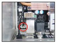
5. This photo shows the LCD Poster installed. Place the device wherever you can monitor the screen.
