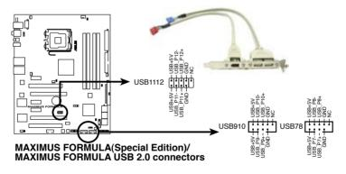
Never connect a 1394 cable to the USB connectors. Doing so will damage the motherboard!
