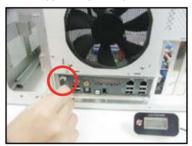
4. Plug the LCD Poster cable into the onboard connector labeled LCD\_CON.
