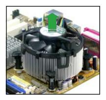
5. Rotate each fastener clockwise to reset the orientation.
