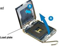
Position the CPU over the socket, making sure that the gold triangle is on the bottom-left corner of the socket. The socket alignment key should fit into the CPU notch
