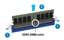
2. Remove the DIMM from the socket.
