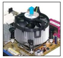
Rotate each fastener clockwise to ensure correct orientation when reinstalling.
