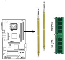
P5KPL-C 240-pin DDR2 DIMM Sockets
