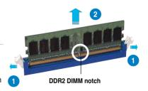
Remove the DIMM from the socket.
