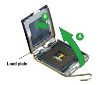
Position the CPU over the socket, making sure that the gold triangle is on the bottom-left corner of the socket. The socket alignment key should fit into the CPU notch.
