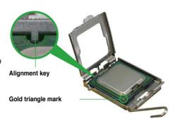
6. Close the load plate (A), then push the load lever (B) until it snaps into the retention tab.
