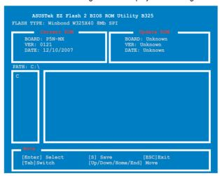
(2) Enter BIOS setup program. Go to the Tools menu to select EZ Flash 2 and press <Enter> to enable it.
