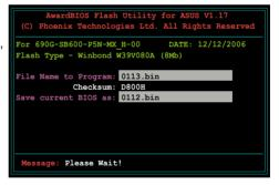
The utility saves the current BIOS file to the floppy disk, then returns to the BIOS flashing process.
