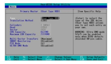
Manually enter the number of cylinders, heads and sectors per track for the drive. Refer to the drive documentation or on the drive label for this information.
