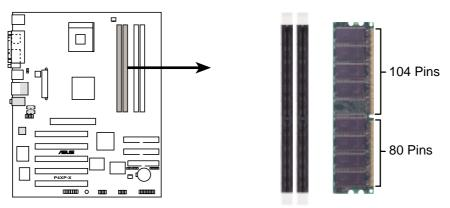
P4XP-X 184-Pin DDR DIMM Sockets
