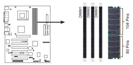
A7V600 184-Pin DDR DIMM Sockets
