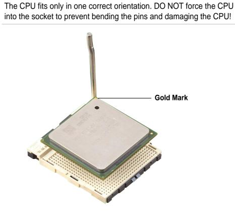
5. When the CPU is in place, press it firmly on the socket while you push down the socket lever to secure the CPU. The lever clicks on the side tab to indicate that it is locked.
