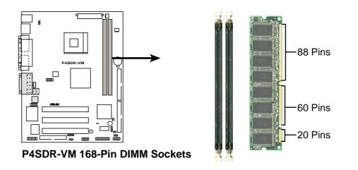
A DIMM is keyed with a notch so that it fits in only one direction. DO NOT force a DIMM into a socket to avoid damaging the DIMM.
