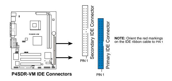
For UltraDMA/133/100/66 IDE devices, use an 80-conductor IDE cable. The UltraDMA/66 cable included in the motherboard package also supports UltraDMA/100.
