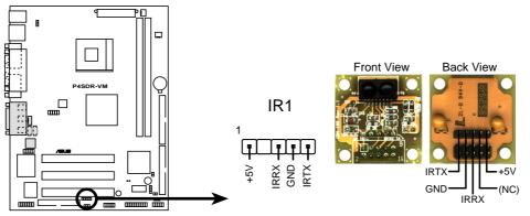
**P4SDR-VM Infrared Module Connector**
