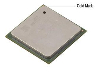
Note in the illustration that the CPU has a gold triangular mark on one corner. This mark indicates the processor Pin 1 that should match a specific corner of the CPU socket.
