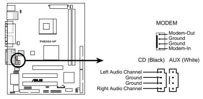
**P4S333-VF Internal Audio Connectors**
