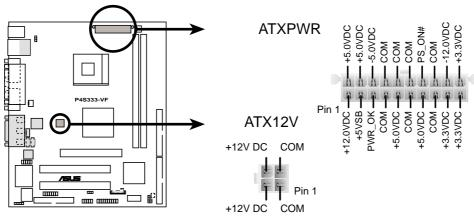
P4S333-VF ATX Power Connectors
