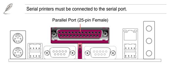
Serial Ports (Teal/Turquoise Two x 9-pin COM1) Two serial ports can be used for pointing devices or other serial devices. To enable these ports, see Onboard Serial Port 1 in 4.4.2 I/O Device Configuration for the settings.
