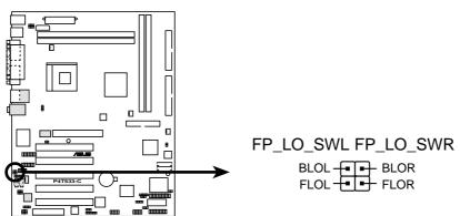
P4T533-C Internal Line Out Connectors
