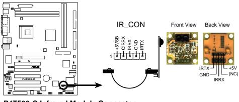
P4T533-C Infrared Module Connector
