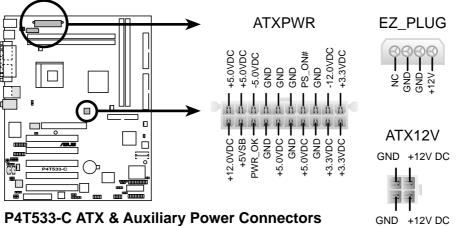
P4T533-C ATX & Auxiliary Power Connectors
