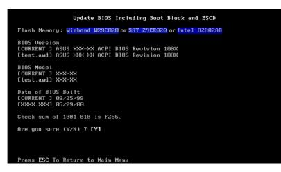
7. The utility starts to program the new BIOS information into the Flash ROM. The boot block is updated automatically only when necessary. This minimizes the possibility of boot problems in case of update failures. When the programming is done, the message *"Flashed Successfully"* appears.
