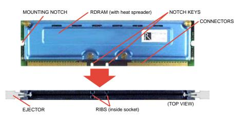
2. With the ejectors in the open position (as shown), push down gently but firmly on the memory module until it snaps into place. The guides on the socket's ejectors should go through the two mounting notches on the module and the ejectors should close. If necessary, push the ejectors inward to secure the module in place.
