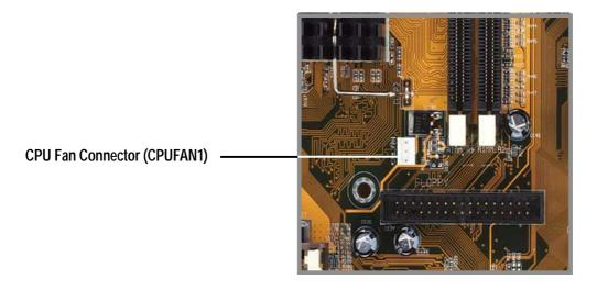
Don't forget to connect the CPU fan connector! Hardware monitoring errors may occur if you fail to plug this connector.
