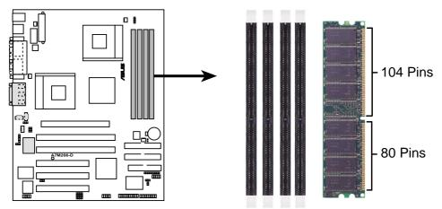
A7M266-D 184-Pin DDR DIMM Sockets
