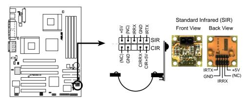
A7M266-D Infrared Module Connector
