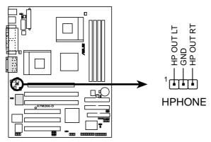
A7M266-D True-Level Line Out Header
