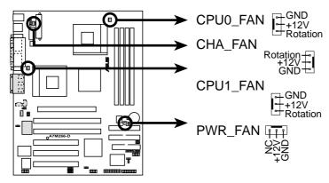
A7M266-D 12-Volt Cooling Fan Power
