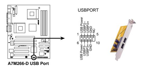
Recommended Setup: Use USBPORT with the bundled 2-port connector set.
