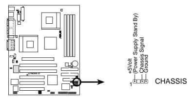
A7M266-D Chassis Open Alarm Lead
