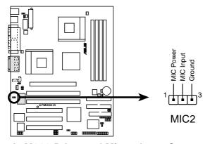
A7M266-D Internal Microphone Connector
