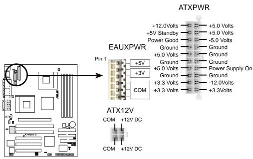
A7M266-D ATX & Auxiliary Power Connectors
