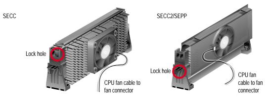
3. If your URM is of type A, make sure the locks are in the locked position as shown.
