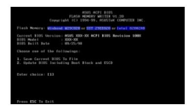
**IMPORTANT!** If "unknown" is displayed after **Flash Memory:**, the memory chip is either not programmable or is not supported by the ACPI BIOS and therefore, cannot be programmed by the Flash Memory Writer utility.
