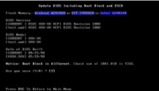
7. The utility starts to program the new BIOS information into the flash ROM. The boot block will be updated automatically only when necessary. This will minimize the chance of a failed updating. When the programming is finished, *Flashed Successfully* will be displayed.
