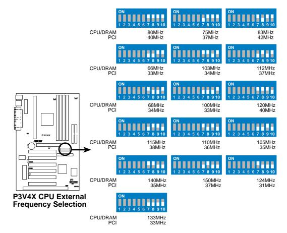
**NOTE:** Overclocking your processor is not recommended. It may result in a slower speed. Voltage Regulator Output Selection (VID) is not required for Pentium III/II processors because they send signals directly to the onboard power regulator.
