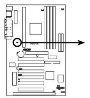
Power Supply Thermal Sensor Connector
