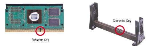
2. Push down firmly but gently the SECC2/SECC/SEPP into the URM until it snaps into place.
