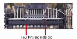
**NOTE:** The SEPP heatsink and fan (for Intel Celeron processors) is similar to the SECC2 heatsink and fan except that the clamping design is different.
