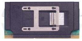
Example of an incorrectly installed retention clip
