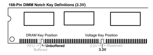
The notches on the DIMM will shift between left, center, or right to identify the type and also to prevent the wrong type from being inserted into the DIMM slot on the motherboard. You must tell your retailer the correct DIMM type before purchasing. This motherboard supports four clock signals.
