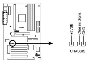
P3V4X Chassis Intrusion Alarm Lead
