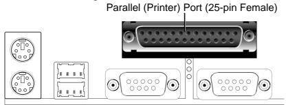
Serial Port COM1 and COM2 Connectors (Two 9-pin male) The two serial ports can be used for pointing devices or other serial devices. See Onboard Serial Port in 4.4.2 I/O Device Configuration for settings.
