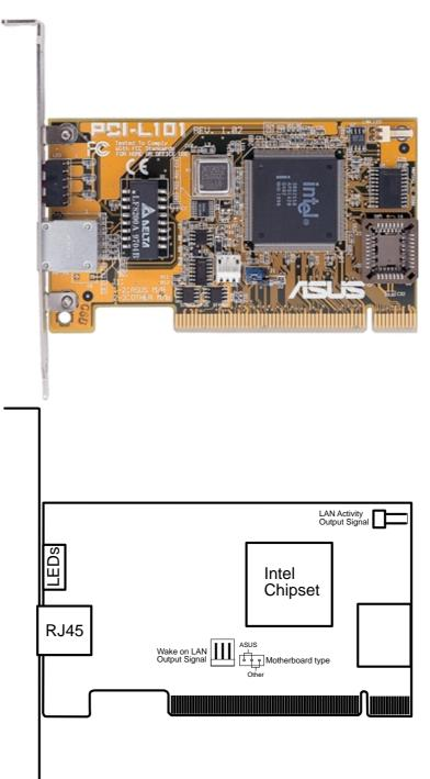
If you are using the ASUS PCI-L101 on this motherboard, leave the jumper on its default setting of "ASUS." If you are using another brand of motherboard, set the jumper to "Other." Connect the Wake on LAN (WOL) output signal to the motherboard's WOL\_CON to utilize the Wake-On-LAN feature of the motherboard. Connect the LAN activity output signal (LAN\_LED) to the system cabinet's front panel LAN\_LED to display LAN data activity.
