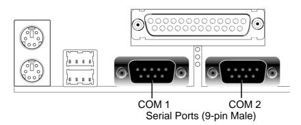
5. Universal Serial BUS Port Connectors 1 & 2 (Two 4-pin female) Two USB ports are available for connecting USB devices.
