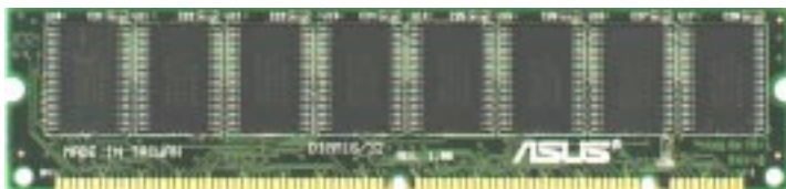
Non-ECC SDRAM DIMM (8 chips)
