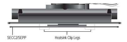
**WARNING!** Make sure the heatsink is mounted tightly against the SECC, SECC2 or SEPP; otherwise, the CPU will overheat. You may install an auxiliary fan to provide adequate circulation across the processor's passive heatsink.
