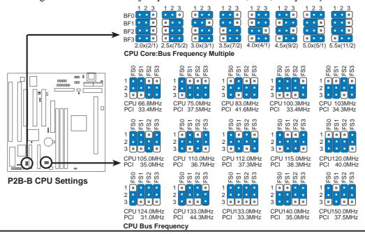
**WARNING!** Frequencies above 100MHz exceed the specifications for the onboard Intel Chipset and are not guaranteed to be stable.
