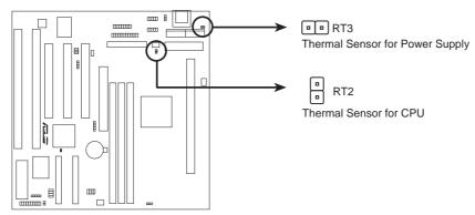
**P2B-B CPU Thermal Sensor Connectors**
