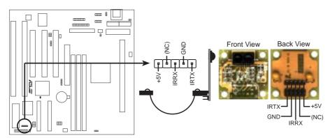
**P2B-B Infrared Module Connector**
