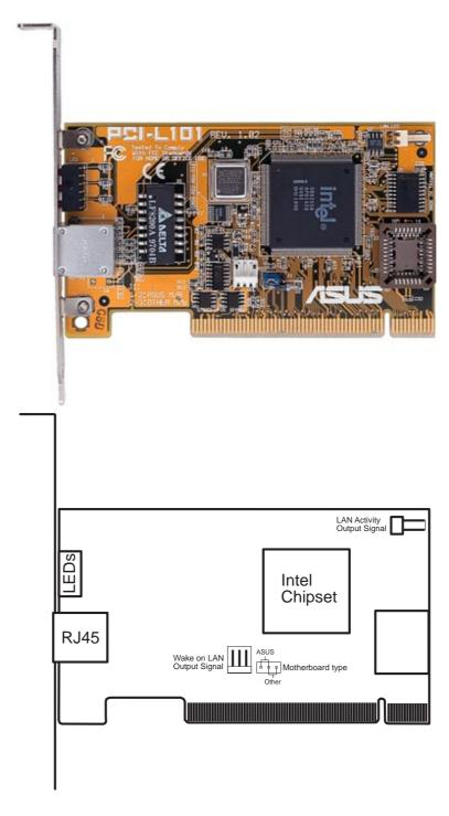
If you are using the ASUS PCI-L101 on an ASUS motherboard, leave the jumper on its default setting of "ASUS." If you are using another brand of motherboard, set the jumper to "Other." Connect the Wake-On-LAN (WOL) output signal to the motherboard's WOL\_CON in order to utilize the Wake-On-LAN feature of the motherboard. Connect the LAN activity output signal (LAN\_LED) to the system cabinet's front panel LAN\_LED in order to display the LAN data activity.
