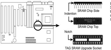
Insert one 16K8 or 32K8 SRAM chip as shown by the Top view with the semicircle "Indention" on the same side as the "Notch."
