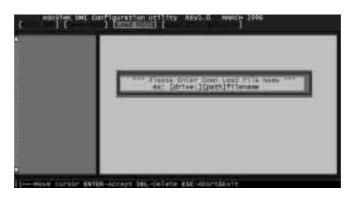
You can load the disk file to memory by entering a drive and path and file name here.
