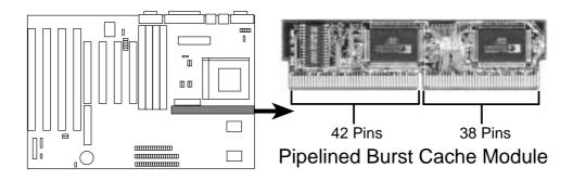
Insert the module as shown. Because the number of pins are different on either side of the break, the module will only fit in the orientation as shown.
