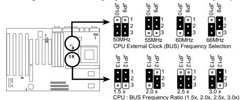
Set the jumpers by the Internal speed of the Intel, AMD, or Cyrix CPU's as follows:
